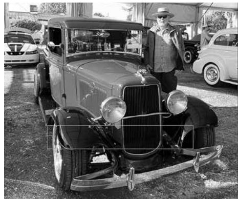
Jerry Klinger's newly acquired 1934 Ford pickup. It has a 350 Chevrolet motor, transmission and rear end. A beautiful truck and a winner at Cutsforth's Cruise-In.
